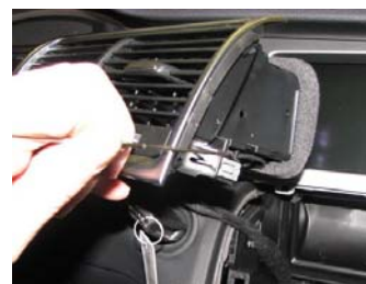
Q7 Air Vent Removal Hole Location
