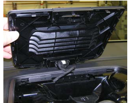
Upper air vent removal
