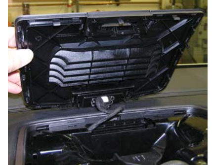
Upper air vent removal
