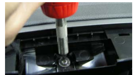
Torx screw to remove shroud
