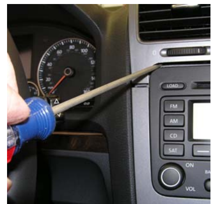
Flat screwdriver pry location to release plastic clip
