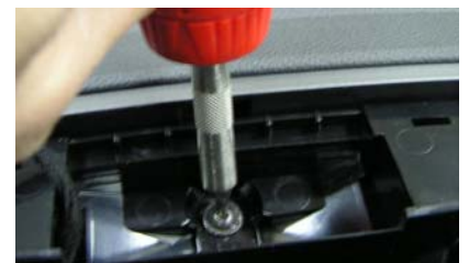
Torx screw to remove shroud
